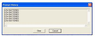
Figure 2-7 Flowlink low-voltage warning
